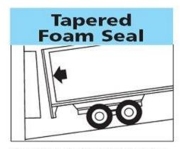
IF AN inclining or declining ramp is a problem, NOVA SEAL offers a solution. Sides of foam seal can be tapered to match the angle of the ramp.
