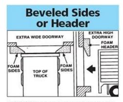
WHERE foam seals cannot be mounted inside doorways, or door frames are too wide or high, beveled foam sides and head pad can be used to seal the gap.
