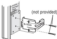
**1.3B** Slide the carriage bolt into the slot on each sensor.
