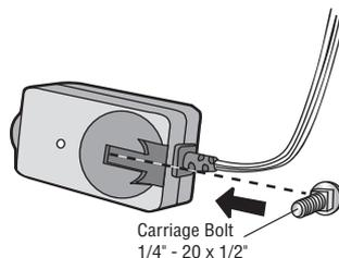
**1.3A** Insert the bolt through the hole in the sensor bracket and attach with the wing nut. The lenses on both sensors should point toward each other. Make sure the lens is not obstructed by the sensor bracket.
