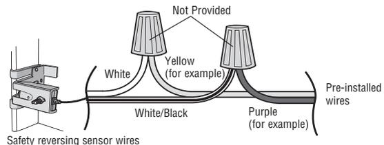
**2.4B** At the garage door opener, strip 7/16 inch (11 mm) of insulation from each end of the wires previously chosen for the safety reversing sensors. Twist the like-colored wires together.
