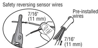
**2.3B** Connect the pre-installed wires to the sensor wires with wire nuts making sure the colors correspond for each sensor. For example, the white wire would connect to the yellow wire and the white/black wire would connect to the purple wire.
