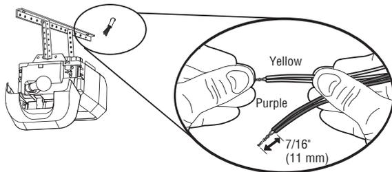
**2.5B** Insert the wires connected to the white safety sensor wires to the white terminal on the garage door opener. Insert the wires that are connected to the white/black safety sensor wires to the grey terminal on the garage door opener.
