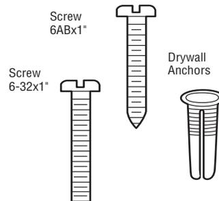
**NOTE:** For gang box installations it is not necessary to drill holes or install the drywall anchors. Use the existing holes in the gang box.
