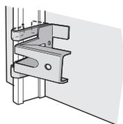
**1.2A** Slide the carriage bolt into the slot on each sensor.
