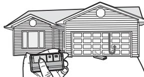
If the door stops and does not reverse on the obstruction, increase the down travel (refer to Adjustment Step 1).
