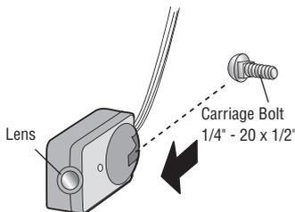
**1.4B** Insert the bolt through the hole in the sensor bracket and attach with the wing nut. The lenses on both sensors should point toward each other. Make sure the lens is not obstructed by the sensor bracket.
